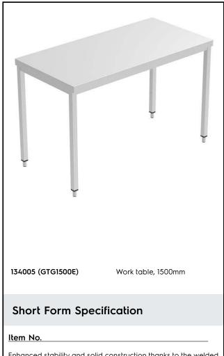
Enhanced stability and solid construction thanks to the welded frame and legs. The 50mm high worktop in 304 AISI stainless steel, with Scotch Brite finishing 15/10 mm in thickness, has antidrip edges and welded corners. 18mm thick undertop reinforced worktop, it's completely waterproof, double-sided laminated and 100% recyclable. Square section legs and height adjustable feet (-20/+30 mm) in 304 AISI stainless steel.
